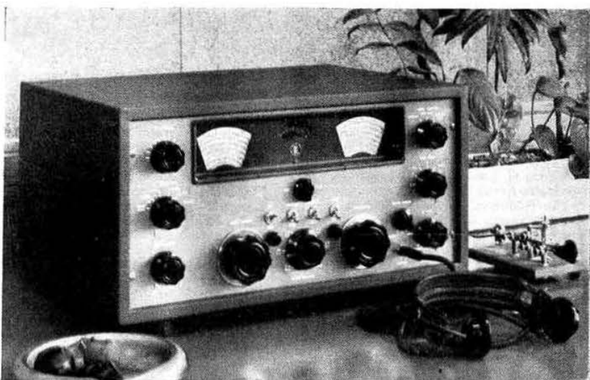
The GPR-90 Communications Receiver measures 20 in. by 10 in. by 15 in. deep and weighs 52 lb. It costs $395.
